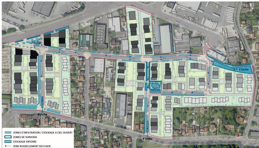
LE VOLUME DE RETENTION TOTAL POUR LA ZAC NECESSAIRE POUR STOCKER LES EAUX ISSUES D'UNE PLUIE DECENNALE EST D'ENVIRON 1298 M.
